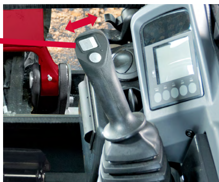
2 Proportional PTO control lever
